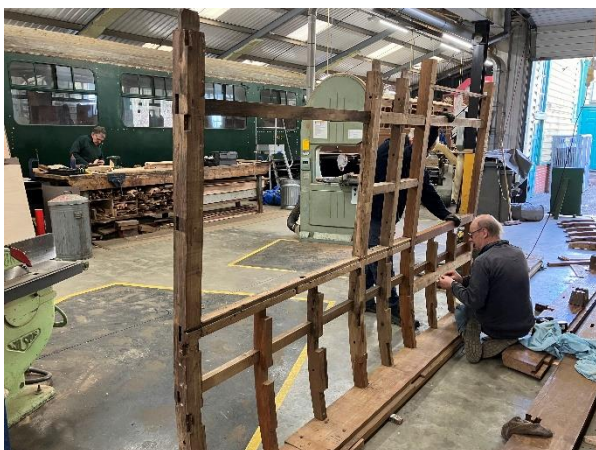
Repaired/renewed frame section 13-22W trial fitted into the new bottom side. 19 Mar 2025
