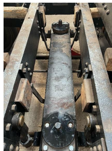
A modified lower bolster plank back in the southern bogie, March 2025 (Stuart Pay). The thickness of the round castings at each end of the plank has been reduced by milling off ½" of metal.
