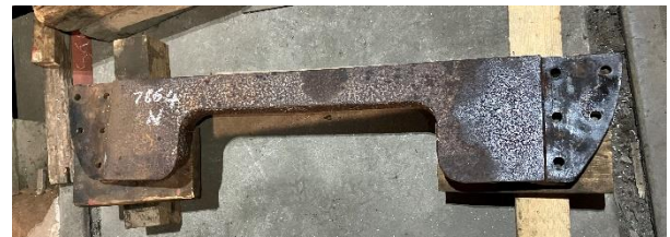
Bottom casting from the north end gangway faceplate. 26 Jan 2025
