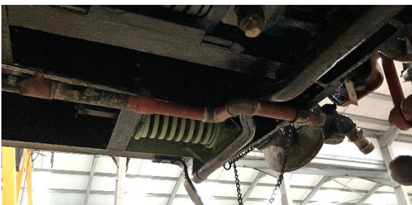
Steam heat pipe south end, modified to increase projection beyond headstock for better clearance. 4 Jan 2025
