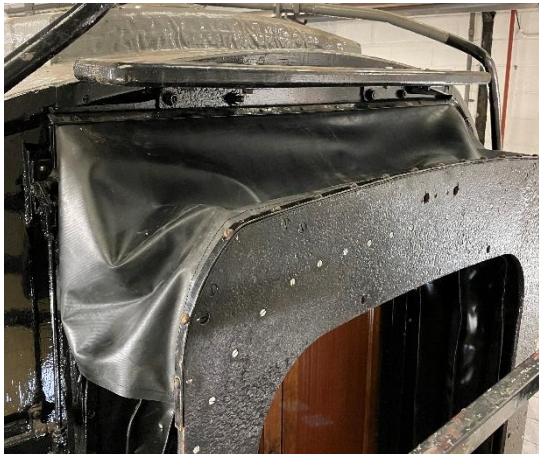
South end gangway bellows connected to the faceplate by the row of machine screws and covered by newly installed cinder guard. 1 Mar 2025
