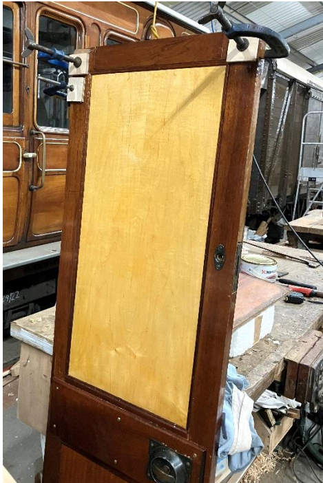
Internal door from 7864 showing the newly applied sycamore veneer. 30 Oct 2024
