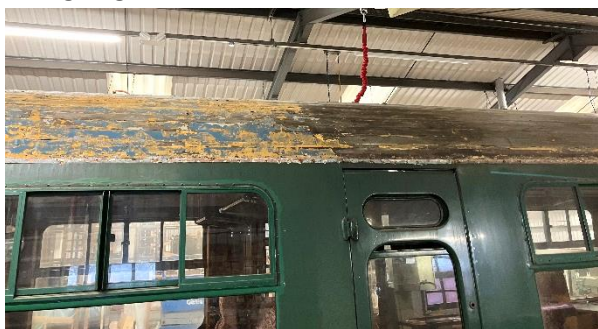
The west side of 1482's roof at the point where the southern half had been cleaned and sanded while the rest still needed attention. 7 Jan 2025
