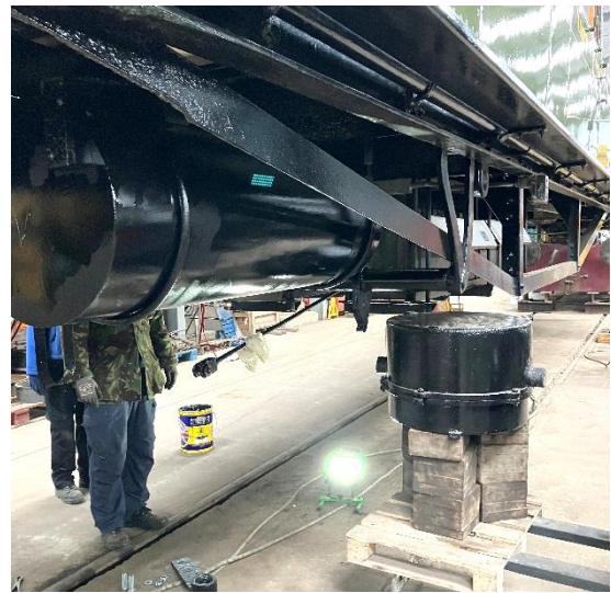
Installing the west side vacuum cylinder, 5 Mar 2025. One of the new reservoirs is on the left of the picture.
