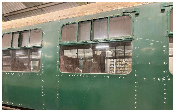
The east side of 1482 showing progress in removing loose filler around screwheads. 26 Mar 2025
