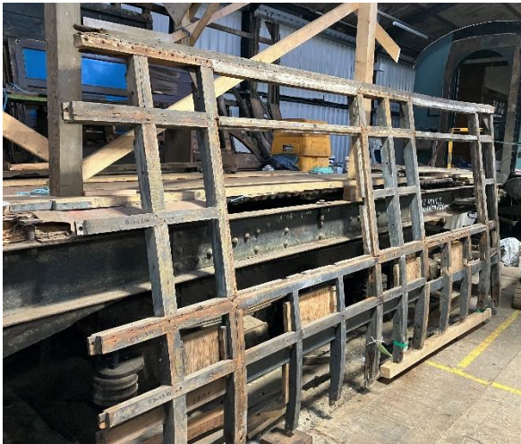
The first section of west side framing to be taken off the vehicle. Pillars 2-12W plus rails A-E and cantrail pictured on 14 Sep 2024.
