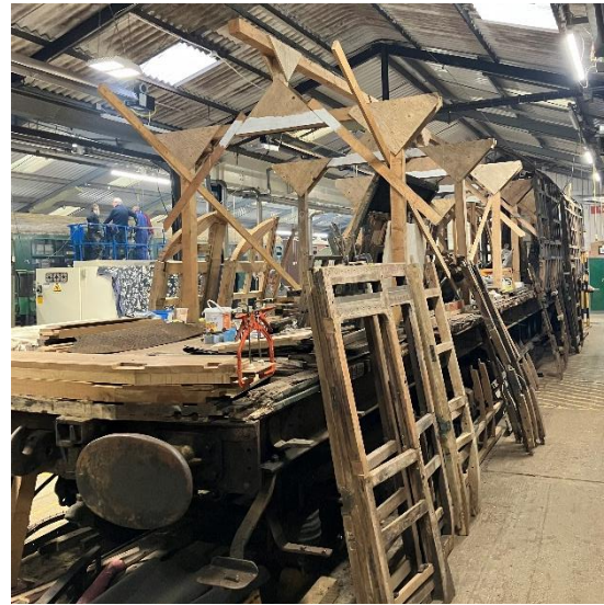
The fully dismantled southern end of 7864, pictured on 8 Feb 2025.
