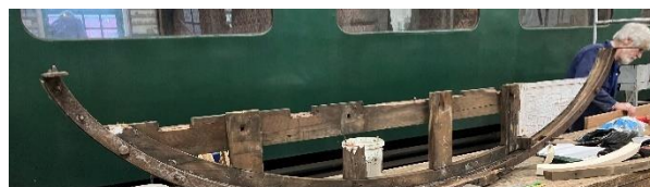
An example of a partition roof hoop; this one divides the north end vestibule from the kitchen. 16 Nov 2024
