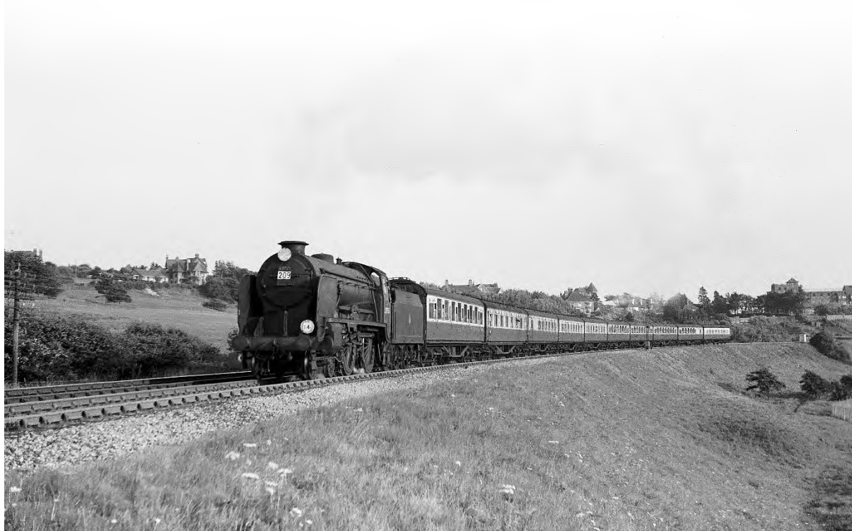
A Schools class 4-4-0 at West St Leonards with a rake of Maunsell Restriction 0 carriages forming the 6.55 pm Hastings to Cannon Street service on 31 July 1955. Photo: Bluebell Museum Archive – John J Smith collection.
