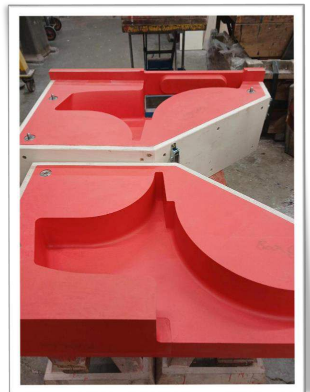
Above: Work on the patterns for Stowe's new left hand cylinder block. Photo: East Coast Castings
