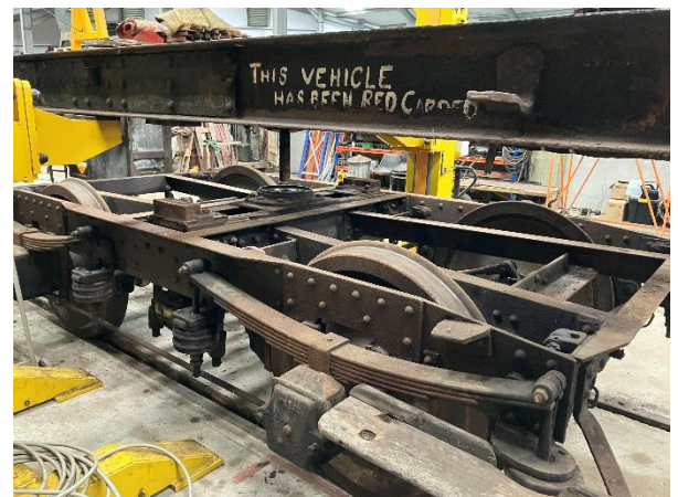
The underframe being lifted clear of the bogies. 20 August 2025
