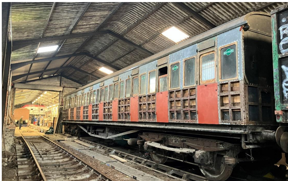
A rare chance to photograph '100 seater' No 971 in Nov 2024. 'A road' was being shunted and so the doors into the works and at the south end were open, letting in some light. Repairs to all of 971's east side doors were finished in August so recently the first of the west side doors was removed for similar repairs.
