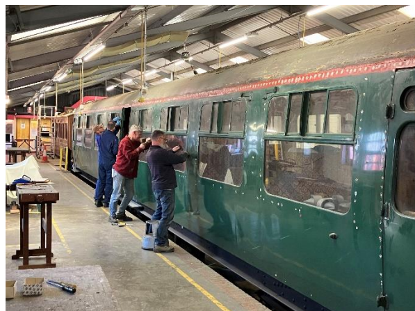
The team working to remove popped filler over the bodyside screwheads. 12 Apr 2025
