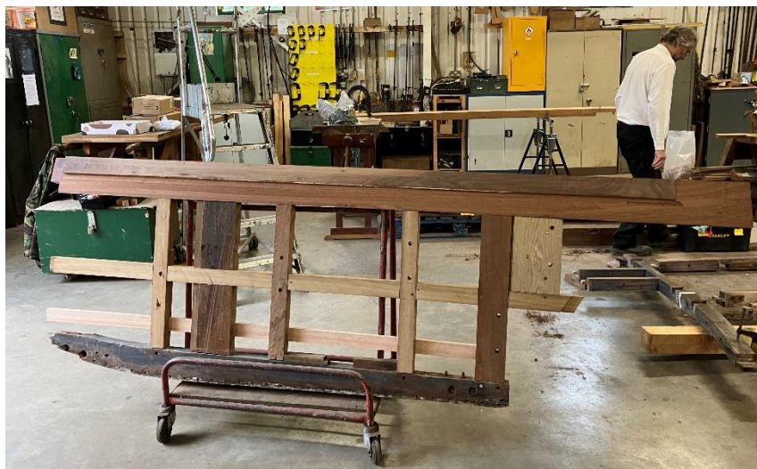
The new north-west end frame fitted to its new crash pillar and trial fitted to the corner pillar, 30 Jul 2025
