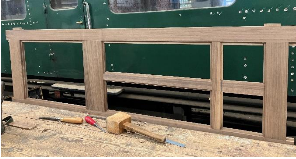
The newly assembled frame for an internal sliding door, made in walnut. 16 July 2025
