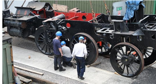
Leading set completed. Driving boxes set to engage.
