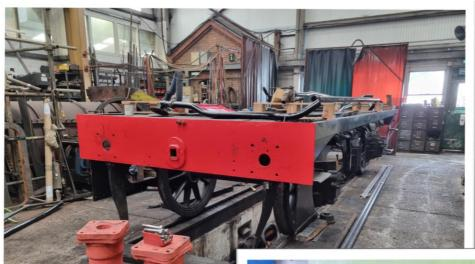
Tender chassis (left) and brake cylinders (below).
