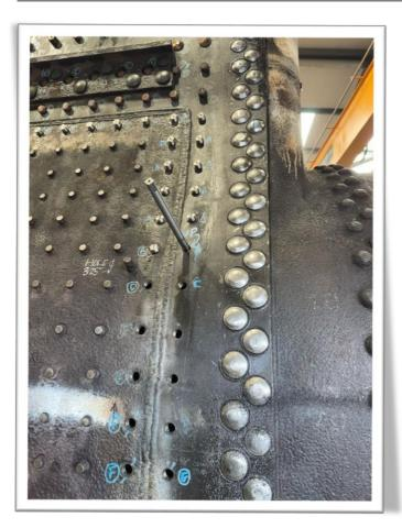
**Left:** Completed copper and monel stays plus tapping the remaining holes on the new outer wrapper. Photo courtesy of Leaky Finders.
