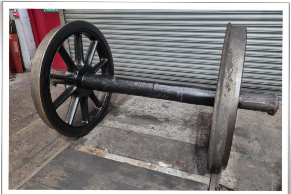
Right: Tender wheel set ready for being re-painted.
