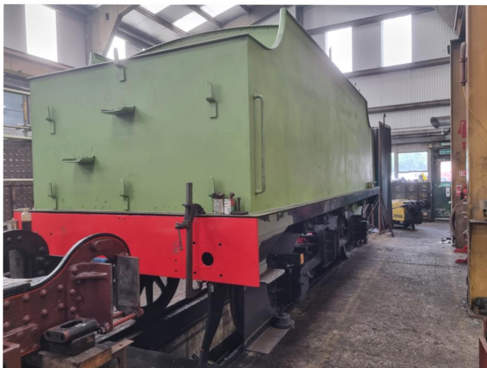
Left: Tender tank and chassis temporarily re-wheeled. Photo – Steve Pilcher
