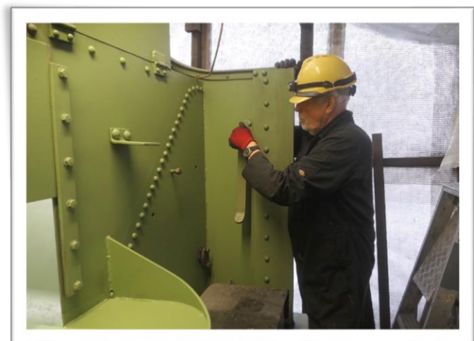
Top: View of outer wrapper of 541 firebox, with patch screws being fitted. Photo: courtesy Leaky Finders
