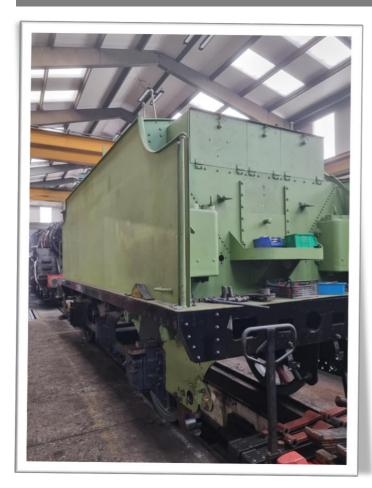
**Left:** Another view of the new tender tank and chassis temporarily re-wheeled.
